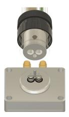
5. Position the filter on the base plate
